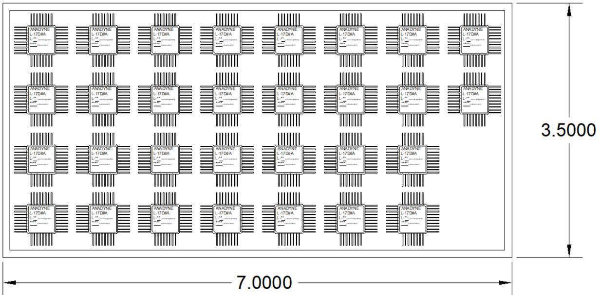
Dimensions in inches. L-17D parts are shipped in conductive plastic packaging with soft conductive foam padding, with up to 30 parts per box in the following arrangement unless instructions are given and agreed upon ahead of time.
