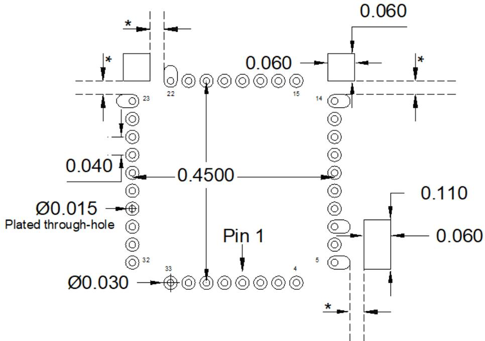
\* Adjust metal ground pad to pin spacing to accommodate bypassing capacitor of choice.
