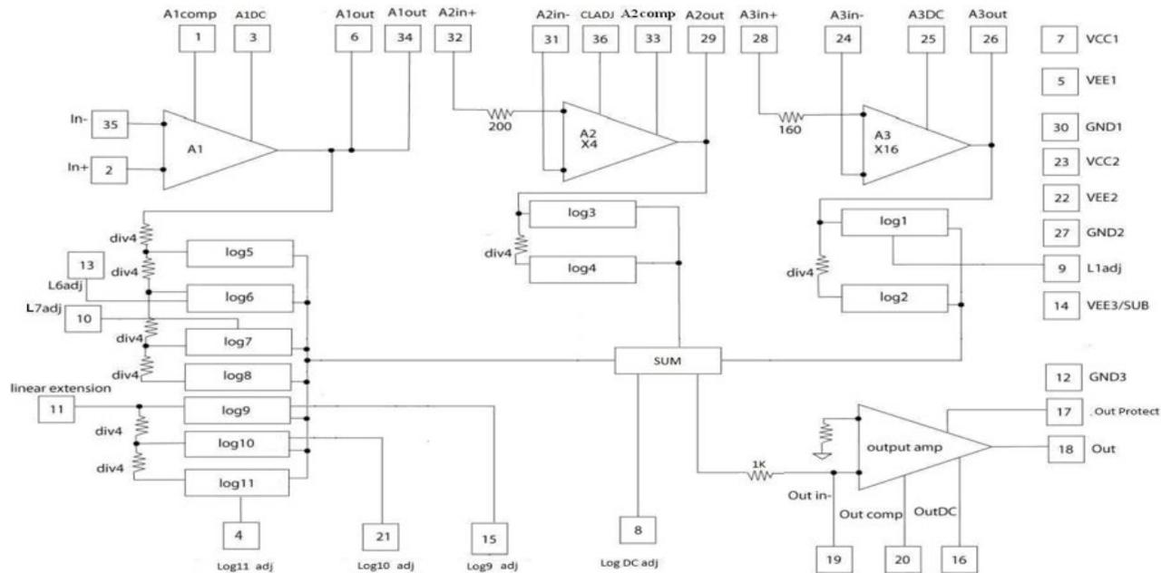
Note: for pinout A: Out Protect and Out are internally connected
