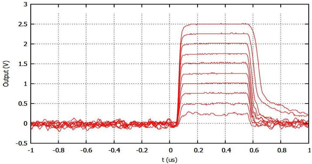
Notes: Pulse ladder has 5 dBm increments between rungs.
